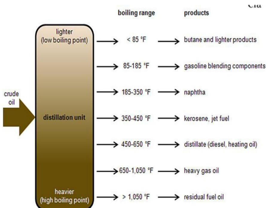
This simplified drawing shows many of a refinery's most important processes.
